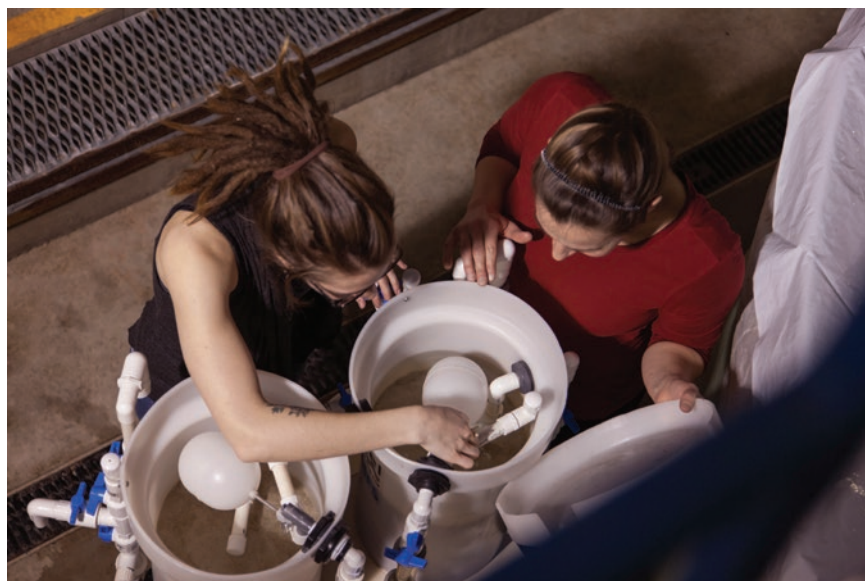
College students Jessica Knoop (left) and Heidi Genesis work on a research project to develop a back-flush slow biosand filter that will remove pathogenic microorganisms like Giardia cysts, Cryptosporidium oocysts and E. coli from water, ensuring that it is safe for everyone to drink.
